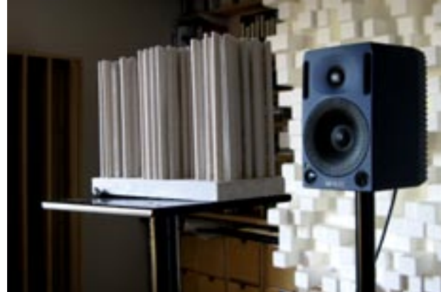
Testing the frequency band 5-10kHz affected by the 1:5 model of the 'Valencia Sonic Lens'
